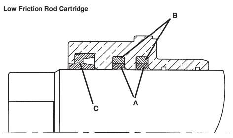
**A** - Dual step-seal rod seals insure positive sealing and smooth operation up to 2,000 PSI.
