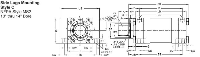
**Note:** Stroke lengths on lug mounted cylinders should not be shorter than the cylinder bore diameter. Consult factory for recommendations on shorter stroke lengths.
