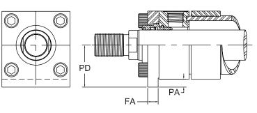
NOTE: A full retainer plate can be included as an option instead of the packing cap on bore sizes 1 1/2" through 6".
