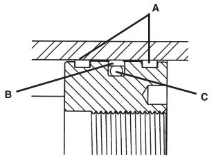
**A** - Dual filled PTFE piston bearings for high load capacity, low friction and no metal-to-metal contact.
